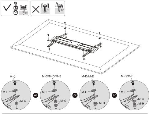
Note: Choose the appropriate screws, washers and spacers (if necessary) according to the type of screen.
