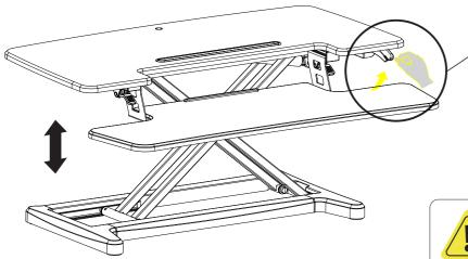
Based on the actual usage, press the handle on one side, and adjust the workstation to the proper height
