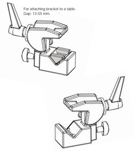
For attaching bracket to a pipe.. Gap: 13-55 mm.
